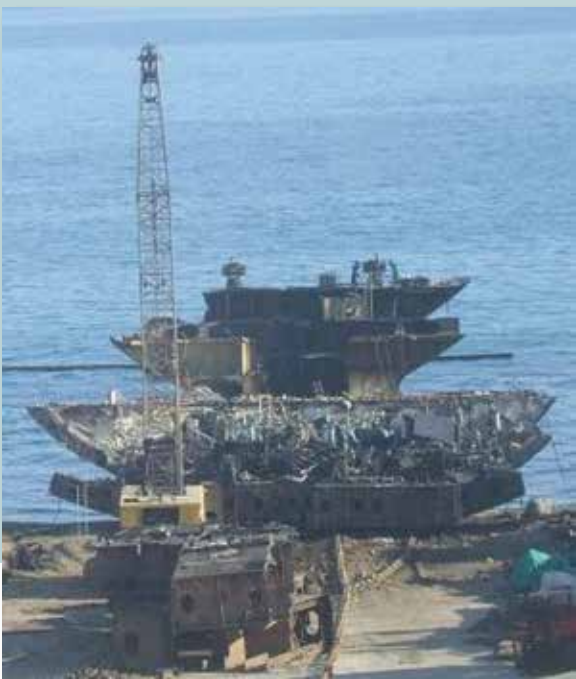
Progress of works 06/06/2013. The remaining part of the keel is winched on to the dry slip way
