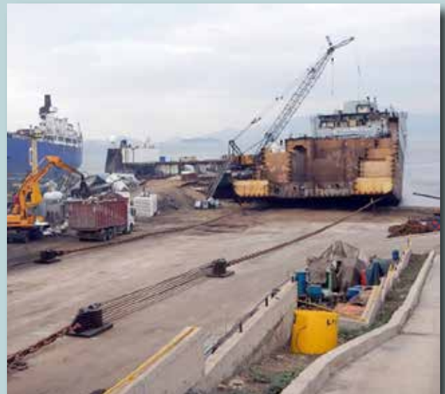
Progress of works 08/11/2012 Dismantling of Top Deck & Accommodation
