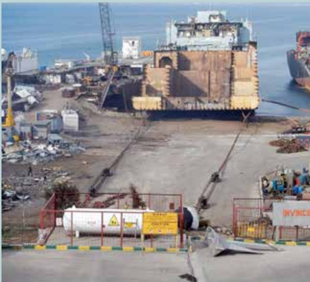
Progress of works 08/11/2012 Dismantling of Top Deck & Accommodation
