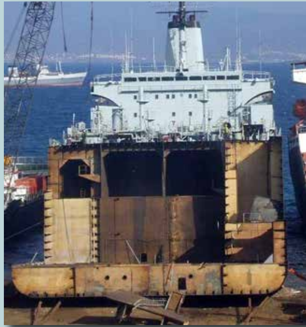
Progress of works (Mid Oct) the ship is now on the Slipway The vessels superstructure and equipment is dismantled while the vessel is afloat, reducing its weight. The vessel is then brought on a dry-land slipway where the keel is dismantled.
