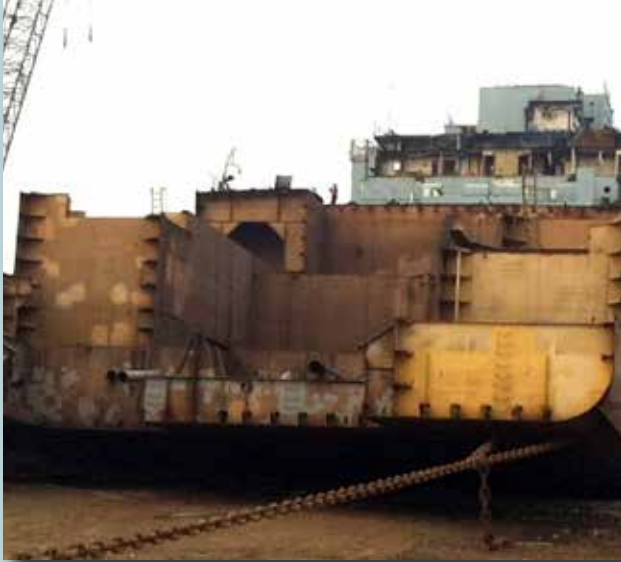
Progress of works 06/11/2012 The vessel is dismantled from "top-to-bottom" while afloat and from "bow-to-stern" on the dry slipway
