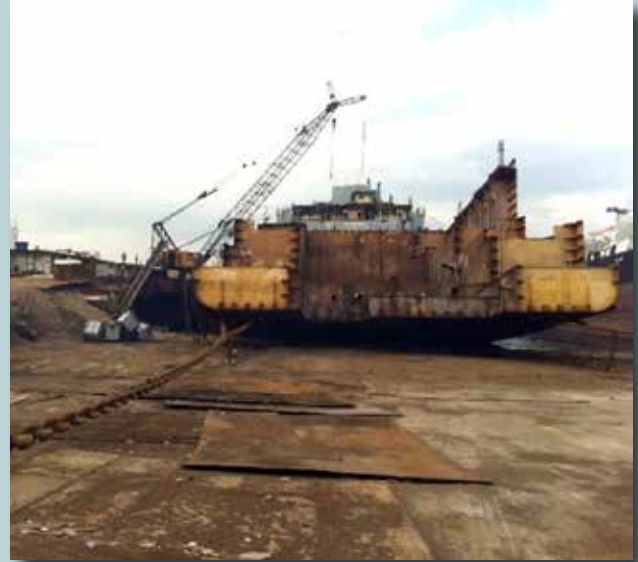
Progress of works 06/11/2012 The vessel is dismantled from "top-to-bottom" while afloat and from "bow-to-stern" on the dry slipway
