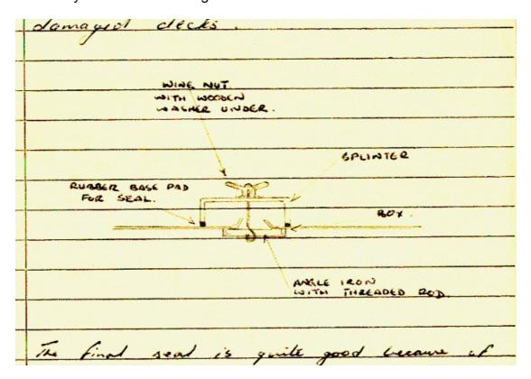
The final seal is quite good because of the rubber base of the splinter box. They come in three main sizes and are suited for most damaged areas up to 1ft square.
