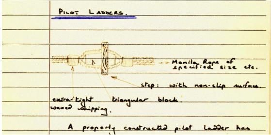
A properly constructed pilot ladder has to conform with set down specifications which describe step length, spacing and the use of proper triangular wooden blocks. Rope size is critical and the use of spreaders to prevent twisting is laid down.
